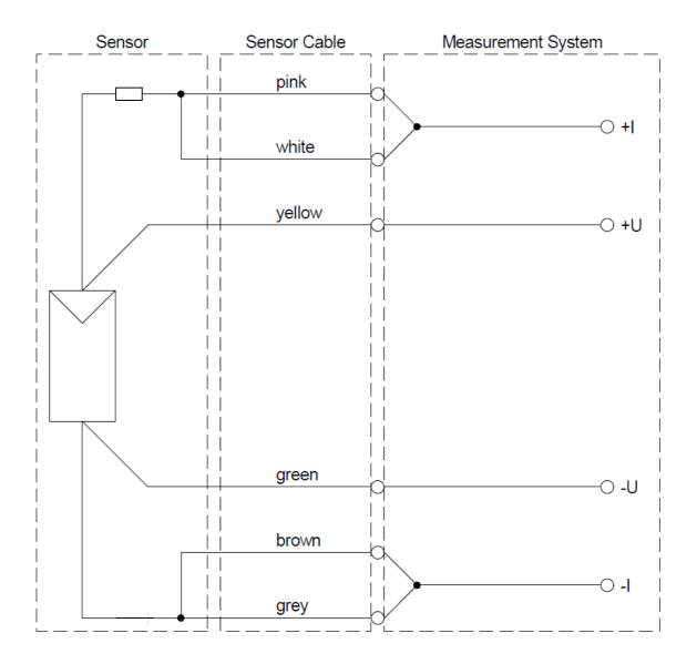
When connected to the external measurement system the current lines shall always be run together (pink and white line for +I and brown and gray line for -I).
